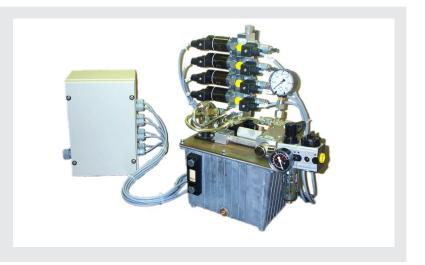
Pump, tank, air regulation unit composing a regulated hydraulic source for single or double-acting hydraulic clamps.
